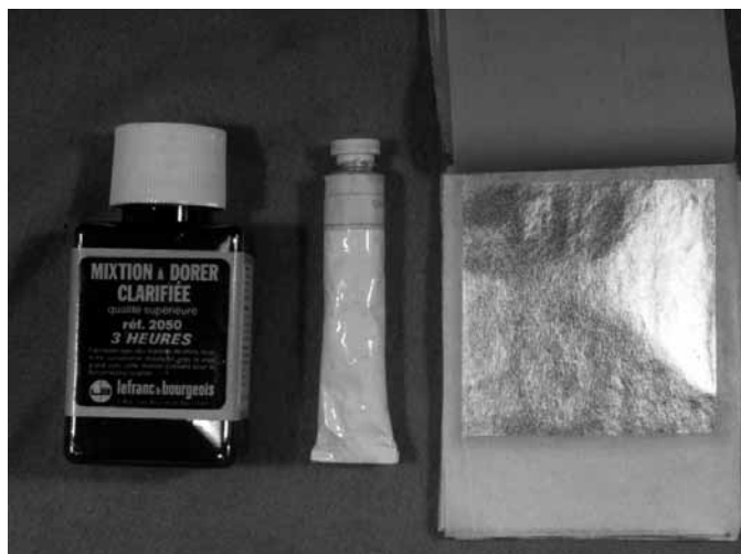
Figure 31. Materials needed for gold leaf application. Left to right, the special slow-drying varnish called gold "size;" yellow or red oil paint, used to color the size; and gold leaves beaten to precise 3.5" squares.
